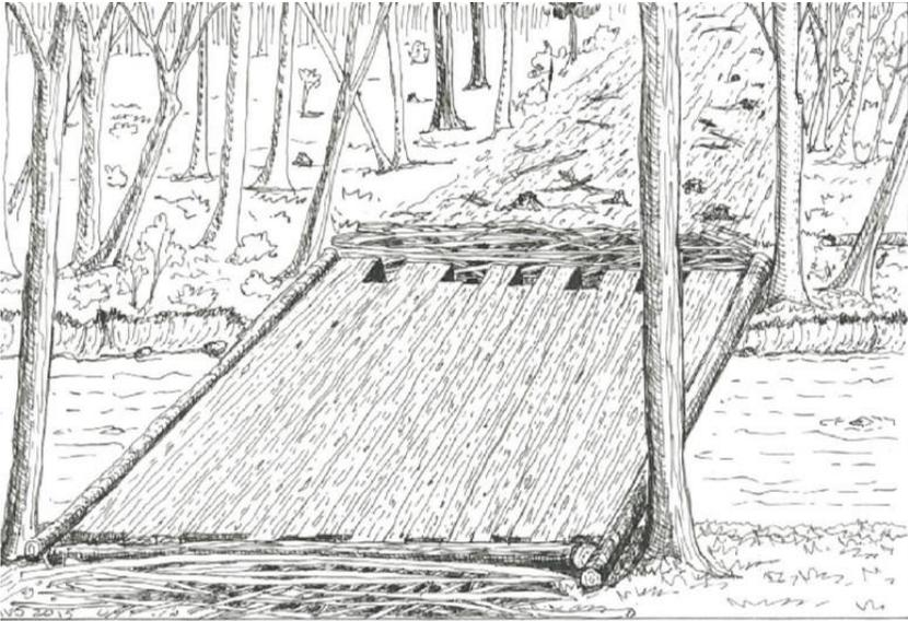
Skidder or temporary bridges are used for crossing streams or other wet low spots. When constructed or set properly they minimize the impact on stream banks, stream beds as well as protect water quality.
