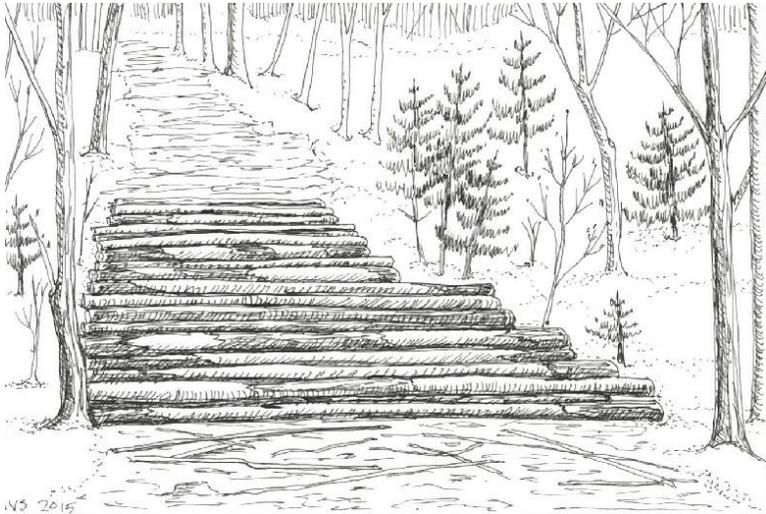
Corduroy is a method of using small logs, poles or slash to cross wet areas which do not have a defined stream channel.
